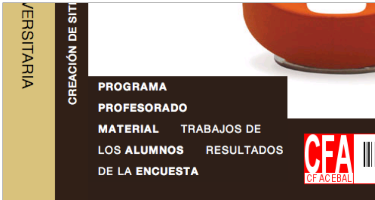
Figure 3. When the browser window is reduced the absolute positioned menu overflows the footer.
